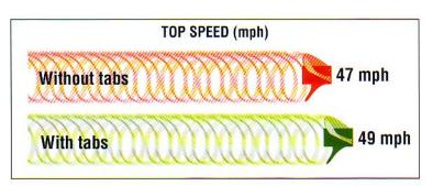
would work. We were also curious as to how they would affect a boat's top speed and fuel efficiency. So we commandeered a 2001 Maxum 1900 SR 19-foot bowrider with a 7-foot, 11-inch beam, 19 degrees of deadrise at the transom and a dry weight of 2760 pounds.
