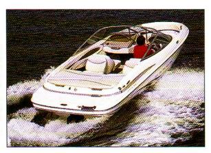
Tearly any planing hull can benefit from a set of trim tabs such as those offered by Bennett or Trim Master. When properly sized and correctly installed, tabs can improve acceleration, eliminate porpoising, level unbalanced loads, smooth out a headsea and generally allow you to fine-tune the ride.
