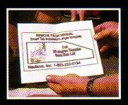
■ STEP 7: To set the angle of the tab, use the template in the owner's manual to create a cardboard jig, reflecting a 25-degree down angle.
