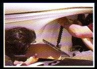
STEP 9: Drill the two holes, countersink each to prevent chipping, apply the adhesive sealant tape, dab the sheet-metal screws with sealant and mount the transom bracket.
