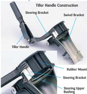
The outboard is designed to turn 90° both left and right of center. This feature helps docking and tight turning of the boat while its 90° stopping points provide an easy-to-recognize refer-
