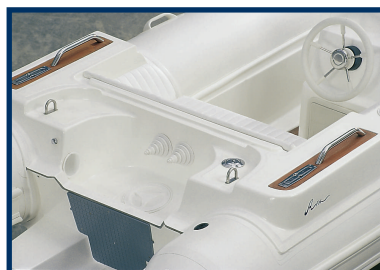
La panca di guida con i tientibene e le bitte a scomparsa in acciaio inox. The driving bench with lifelines and stainless steel pull-up bitts.
