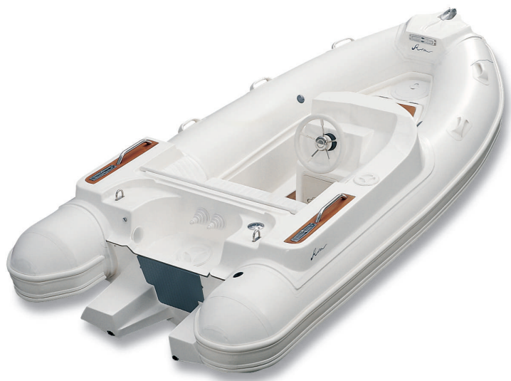
La panca di guida con i tientibene e le bitte a scomparsa in acciaio inox. The driving bench with lifelines and stainless steel pull-up bitts.
